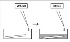
Pipette 700  $\mu I$  wash buffer and 300  $\mu I$  conjugate into each incubation tray with strip.
