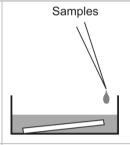
Pipette 10 µl serum sample into the designated incubation trays with sample buffer.
